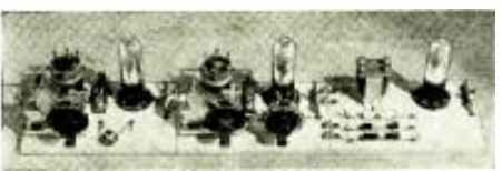
Above is a set-up of apparatus for studying the principle of generation and detection, made by the student of radio. The three units are assembled from the parts shown below.
