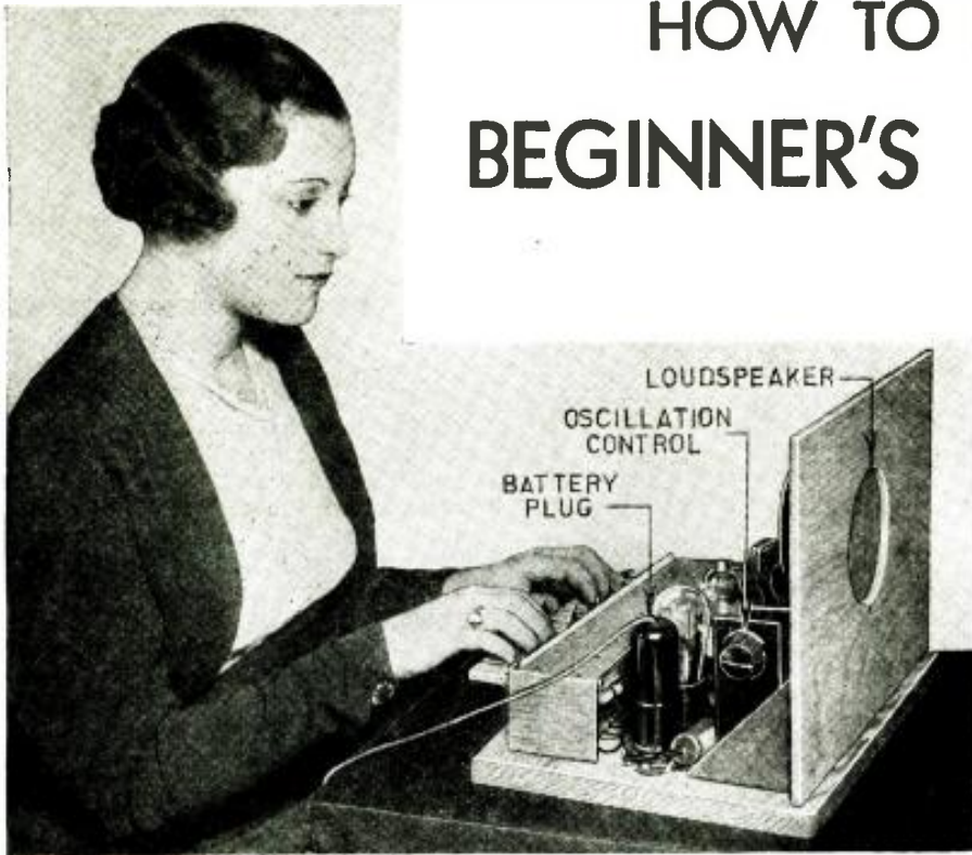
Fig. A The Pianotron in operation. This musical instrument is played like an organ.
