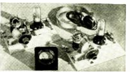
Above is a set-up of apparatus for studying the principle of generation and detection, made by the student of radio. The three units are assembled from the parts shown below.
